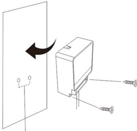
The distance between both screws are 47.5mm.
