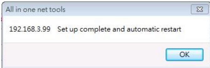
8. Restarted, put off the power line and plug in again. Click the "Search in LAN" button twice and you can find the IP of the equipment. Ensure the internet setting is correct or not.
