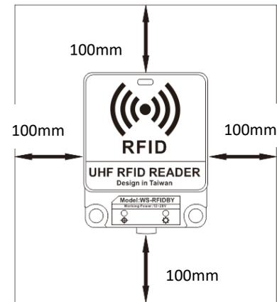
The minimum space room for WS-RFIDBY each side must be 100mm.
