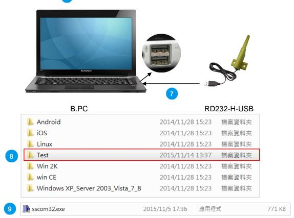
• Open the software, choose your "ComNum" (serial number, "COM3" for example), 10 then choose "9600" for your baud rate 11, and then click on "Open Com" 12 to complete Computer B's setup.
