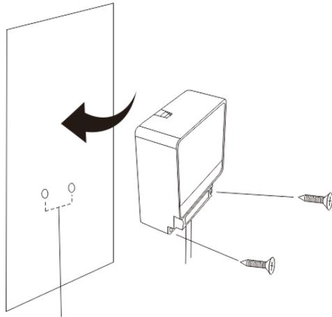
The distance between both screws are 47.5mm.
